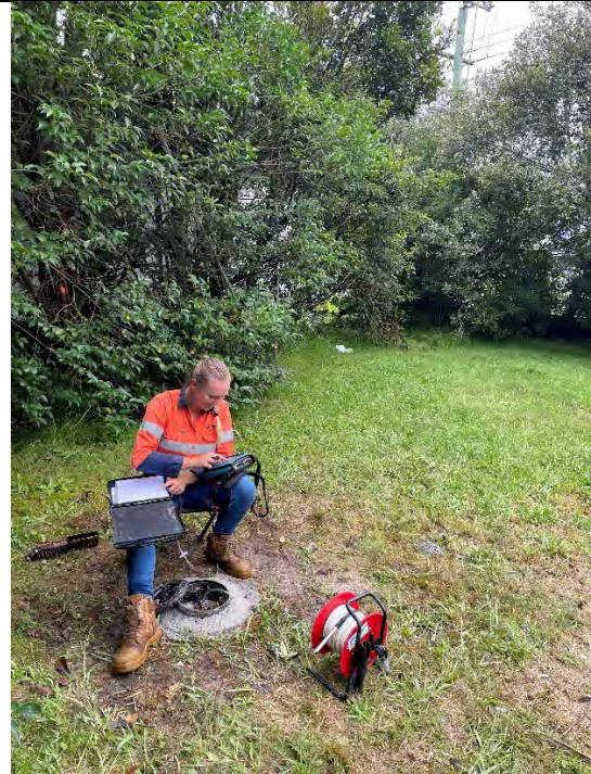
Figure 8. Discrete ground gas monitoring using a GA5000 at GG3.
